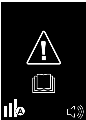
Fig. 17: Component defect indication
